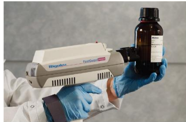
Raman is a flexible inspection technology that is capable of accurate performance scanning both liquids and solids.
